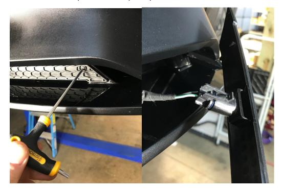
7.- Next take the main light bar power cord and run the power cord through the hole that the oem accessory wire comes through. Then run that new power wire to the back left hand corner of the housing. If you look to the left of the light bar location in the opening, you can shine a light back and see where the power wire will come through on the back side.
