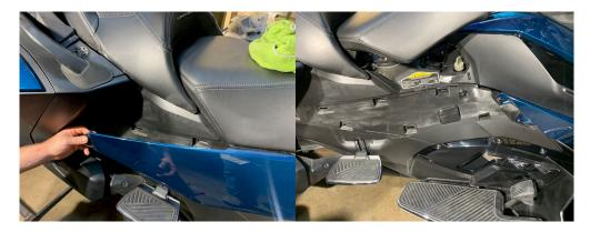
2.-Raise the seat to allow easier access to the docking station wiring. Next remove the upper blue panel shown below. Remove the 3 Torx screws shown. Then remove the 3 push pins under the front trunk.
