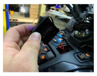
11.- The Light Bar wires plug into the ground wire on the switch and the open terminal as shown below on the left photo.
