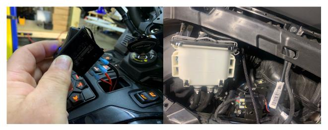
6.- Next remove the front panel shown below. Keep the two screws. Locate the factory accessory wire and keep it out in the open. Remove the plastic panel from the oem connector.
