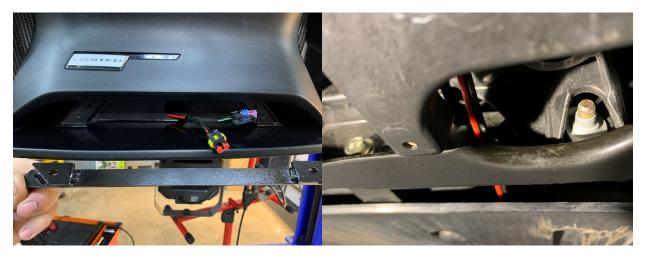
9.- Next Install the Light Bar with the two screws provided. Adjust the light bar so the light point level. You may adjust it to your specific needs.
