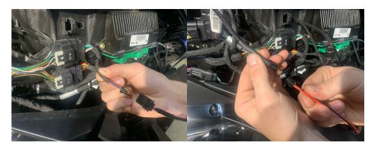
10.- the remaining plug on the accessory harness put that plug back in the existing plug resting hole.
