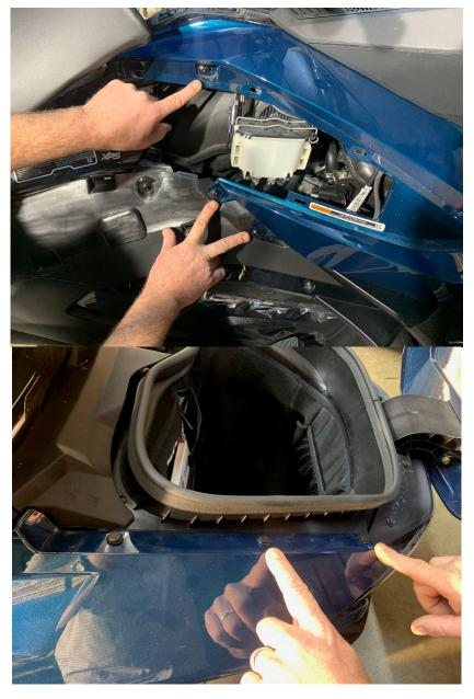
6.- Then remove the upper blue panel by pulling the panel away and sliding forward towards the front of the Spyder to release the panel.
