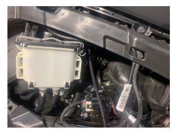
9.- The kit comes with the accessory power wire that plugs into the Factory Accessory wire as shown below on the left. Plug the supplied accessory wire into the factory plug as shown below. Then plug the other accessory end into the docking station plug as shown on the photo below on the right.
