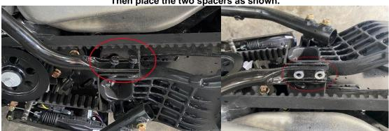
6.- Locate the two frame bolts here. Remove these bolts. Then place the two spacers as shown.
