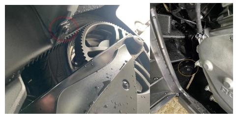
Notice these two photos of the bolt on the left underside and the screw on the right photo circled in yellow to be removed.
