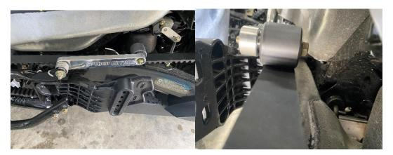
8.-Your new RT belt Tensioner is now installed. Now for the fun part, in reverse reinstall all your panels. Be sure to work the panels in place with caution.
