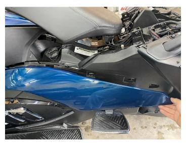
3.- Once removed next remove the driver and passenger footrest. This will make the removal of the large black panel easier without the risk of damaging it or its fasteners.
