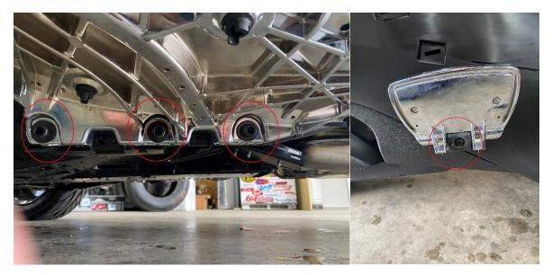
4.-Next remove the black panel the upper push pins and other bolts as shown below.
