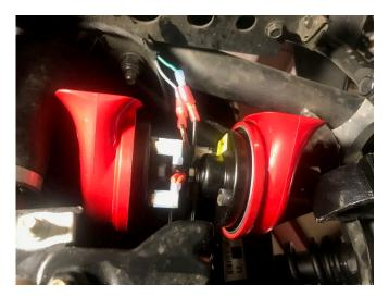
8.- Take the wiring harness and connect the ground terminal next the relay to the ground post on the battery and connect the red fused wire to the positive battery terminal.
