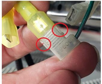
Then connect the pairs of horn wires to each horn. Again, it makes no difference which connector for each horn is on what terminal. No polarity to deal with. They are grouped in pairs, so each pair connects to each horn. Tie the new harness to the frame area with the new wire ties.
