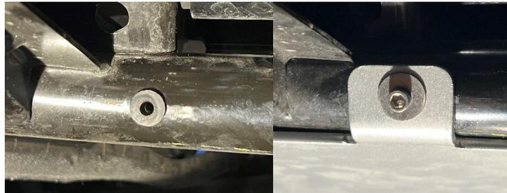
3.- Next take the Skid Plate and locate it under the Ryker with the rear of the skid plate aligned with the two mounting tabs on each side as shown below. Install the supplied screw. Do the same for the opposite side.
