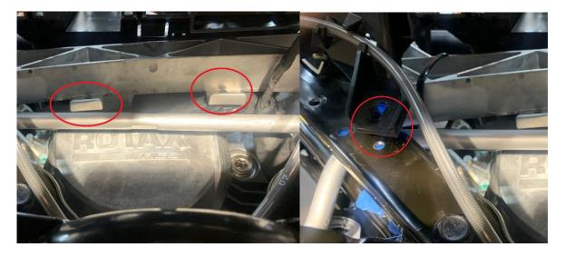
8.- Take the new way bar as shown below and run it through the left side rectangle hole. The bar should be located as shown with the end bent tabs in the upward position. With the left lower shock bolt removed it will be easier for you to allow the end of the sway bar to be moved around as shown on the lower right photo.
