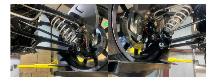
6.- Once the factory sway bar and bushings are removed, as shown below take blue painters' tape and tape up the edges of the side openings and a piece on the right as shown. Do this each side.
