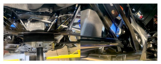
10.- Then install the sets of Sway Bar bushings using the factory bolts. The bushings go in one direction only. The top of the bushings has chamfered cuts to allow them fit in the upper frame channel. Notice the bushing is in two parts you want the hole that is angled to be towards the back with the thicker side of the bushing facing the front of the Ryker as shown below. Do this on bolt sides. Do not tighten down all bolts until all bolts are in their locations.
