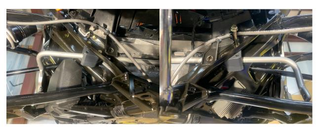
10.- Last step is to reinstall the sway bar links to the sway bar ends. Follow the instructions for the links. Do this for both sides. Notice the bend of the sway bar is downward at the link connection.
