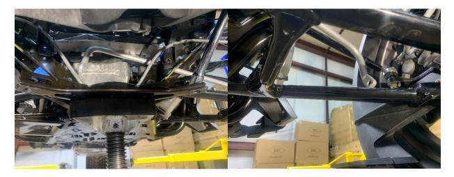
9.- Then take the bar Tilt upward then guide through the right-side rectangle hole as shown below. Once the bar is in this position as below on the right photo form the front push down on the sway bar while pushing the bar to the right side into its final location. Note the angled bend in the sway bar that allows you to fish the bar through the openings.
