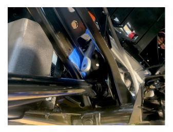
7.- Then the wiring harness below and cut the two wire ties and place the harness under the tabs in red. After you reinstall the new sway bar go back and place the harness back in the slots and use wires to tie up. Remove the two lower and upper bolts holding the plastic radiator frame to the main frame shown below on the right side. Lift this section up as it will help. Shown in red circle on the lower right photo.
