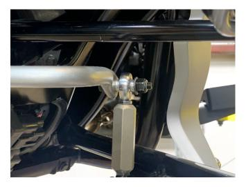
11.-Now reassemble the Ryker in reverse of how you took it apart. Be sure to relocate the bolts in the inter plastic radiator housing. Then lower the radiator back into the position and bolt back as before. Reinstall all shock and lower a-arm bolts to the factory spec. Reinstall the Front Plastic Grille Protector and your Sway bar kits is installed.
