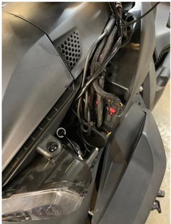
Remove the Left side panel as shown by removing the push pins connectors
