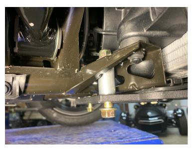
2.- Take the Supplied 3/8" bolts and place the supplied spacer as shown above. The spacer is located between the skid plate of the Grille Guard and the angled slotted gusset brace each side of the frame. Install the washer on top of the frame then the locknut.
