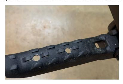
2.- Take the two 5/16" Socket Head Bolts and place the floorboard main support over the footrest and take the mount lock plate and mount it from the bottom as shown below. Screw the bolts down evenly through
