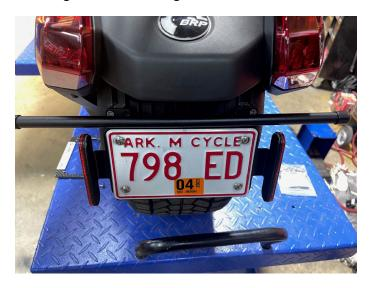
4.- Once installed you can take the flag, remove the two socket had bolts from the bottom of the mount and then place the flag on the mount shaft as shown below. Slide the flag over to the rubber end cap. Tighten down after you have located the flag at the angle you like best. Tighten down and your flag and your flag kit is installed!
