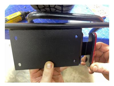
3.- Then take the license plate while holding each reflector and use the four supplied bolts and screw them to the flag mount left & right brackets using the bolts holes in the center of each bracket.
