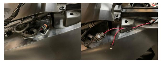
4.- Next take the male plug form the Ryker Docking station and plug into the matching connector as this will supply the switched power to your docking station. The remaining wire end plug is for additional Ryker Factory Accessories.
