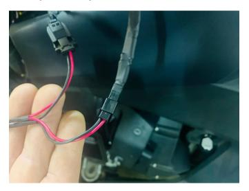
5.- Then tie up the additional wire with supplied wire ties and reinstall the upper front cover. Make sure you leave enough wire from the Docking Station to allow the steering to move full direction each side.
