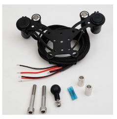
4.- Use the two blue connectors supplied then crimp to the SRT-1U12S power red and black wire and to the positive and negative from the factory wiring accessory wires. Be sure to connect positive to positive and negative to negative. This factory accessory wire is already fused at the fused box.
