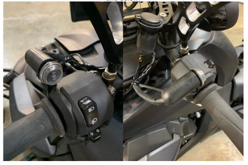
4.- Remove on the left-hand module the upper Torx screw. Place the switch unit in this location and reinstall the Torx Screw This install should look like photos above. Once complete the switch is installed. This provides easy access to the switch like your high beam switch.
