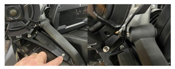
3.- First install the main power wire to the battery with the connector ends at this upper panel area terminal ends to the battery. Remove the front trunk to access the battery. Take the two supplied amp boxes, the Low-level filter and wiring harness and locate them in the upper left-hand panel shown below where the OEM Accessory wire is located. Use the supplied wiring diagram and connect the speakers to
