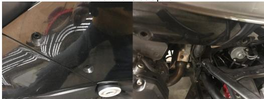
3.- Remove the rear existing Factory Foot Rest 4.-Insert the black Nylon MD spacer in the Rear Foot rest cradle.
