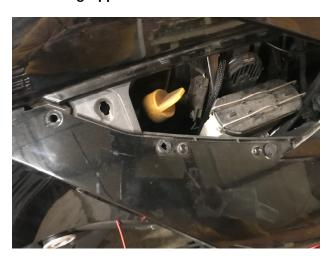
2.- Remove the two bolts each end of the right-side Panel and then remove the panel.
