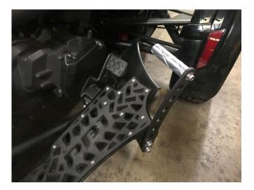
7.- Next take the existing brake pedal pad off the brake pedal arm. Remove the two bolts from bottom side. Take the supplied spacer and new bolts and add the spacer between the brake pedal pad and the brake pedal mount. Secure using the two longer bolts.
