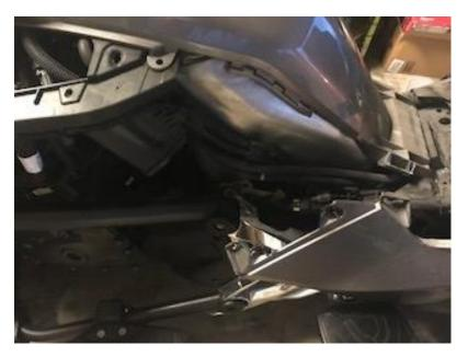
3.-Remove the lower left push pin connector then Lift up the lower panel which allows it to hang freely away from the frame.
