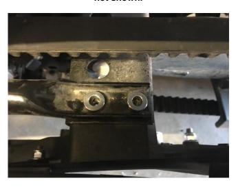
3.-Place RT Idler over the two spacers first adding the right-hand bolt and washer. With supplied new bolts, add medium strength LocTite to both bolt threads before installing. Be sure to press down on the arm at the bracket connector location to level out the mounting bracket to allow the right-hand bolt to align with frame hole. Tighten down right-hand bolt to a snug position. Then remove the 8mm alignment set screw from the left hole and replace with the bolt and washer as shown below.
