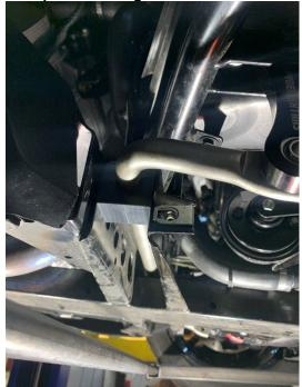
Insert the new sway bar reverse of how you removed the existing. Be sure to take note of the location of the sway bar bushings. Using the supplied grease, grease the inside of the bushings then install the new bushings in the exact locations as the factory installed bushings. Insert the existing bolts and tighten down the nuts holding the bushings in place.
