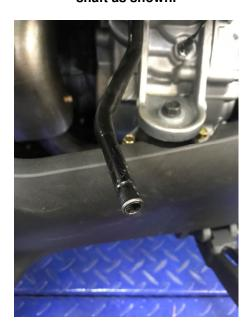
3.- Install the Shifter on the shifter shaft. Then use the new Socket Head Bolt and install the bolt. The shaft at the end is tapered to a larger shaft. The shifter is designed to be tightened against the taper locking it in place. Once tightened it will remain in the location you selected.
