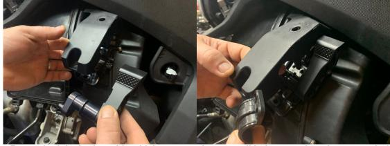
7.-Reattached the brake cable which may require you pull it downward to place over shaft.
