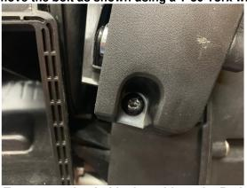
3.- Then remove the T-30 Torx screw that holds the cable to the Brake Lever as shown below.
