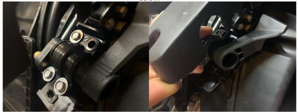
5.- Then remove the Brake Lever from its cradle.
