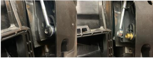
4.-Then lift the cover and using an 8mm socket. Remove the 4 bolts holding the plastic cover over the Brake Lever Shaft. We removed the first bolt in the photo. Then remove the Shaft Cover as shown below.
