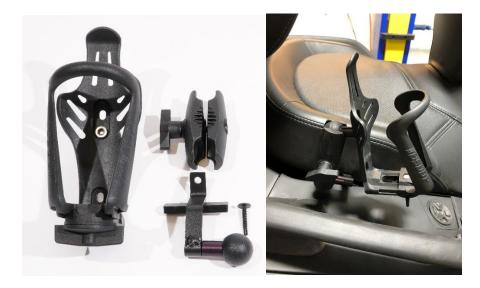
1.- First remove the rear passenger seat. Locate the side rear black panel screw on either side of the RT that you want to mount the holder as shown below. Remove it and take the holder base mount and install back in the same screw hole using the factory screw. The cross bar should mount flat against the panel as shown to support the lower bracket. Tighten down but do not over tighten as this is a plastic mount the screw screws into.
