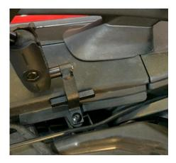
2.- Then adjust the cupholder to fit your needs as shown above. This kit allows many mounting options that will fit your needs. Reinstall the passenger rear seat. Adjust the cupholder as needed.
