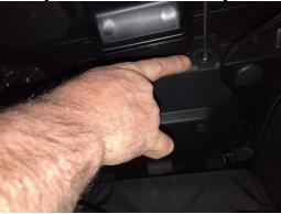
2.- Remove the access panel under the RT allowing access to the horn location. There will be Push Pins to remove.
