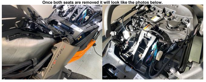
9.- Run the rear portion of the wiring harness along the side of the gas tank wiring existing harness behind the panel shown above. Once the left and right rear speaker connection cable are under the passenger seat area the next step will be to add the speakers. The rear speakers are mounted on a custom-made mounting bracket. There
