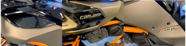
2.-Once the upper panel and the left main side panel are removed the upper panel is where the main wiring harness for the audio system will be routed and the Led light controller for the speakers will be located. Take the main harness with the end that connects to the amp unit that mounts in the front trunk fold the wires over and tape down temporally and fish it down through this space to come out as shown on the location below.
