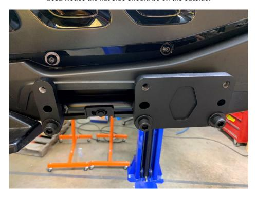
3.- Next take the supplied new bolts and washers and reinstall the Floorboards in the top holes of the new riser blocks. Use Blue Loctite on all bolts. Tighten down all 3 evenly. Do this for the other side as well.
