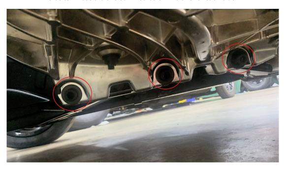
2.- Once removed take the new riser blocks as shown and mount them to the frame. These risers allow the Floorboard to be mounted in 1" increments of rise for a total of 2". Decide on which height fits you best. Notice the flat side should be on the outside.
