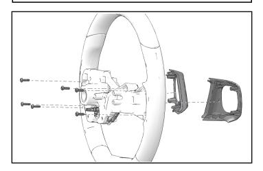
2. Install paddle shifter rear steering wheel cover ④ onto steering wheel. Make sure four clips are in place.
