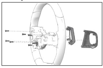
3. Disconnect wiring harness from left-hand (A) and right-hand (B) steering controls.
