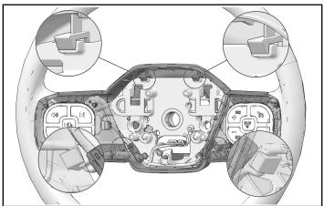
2. Remove and keep six screws and two bezels from steering wheel.
