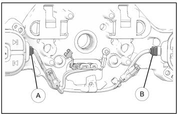
4. Remove two wiring harness fir tree clips (A) and (B) by pushing them out from the rear of the steering wheel. Discard harness.
