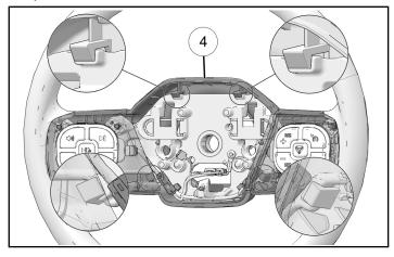
3. Make sure wiring harness ③ is routed as shown.
