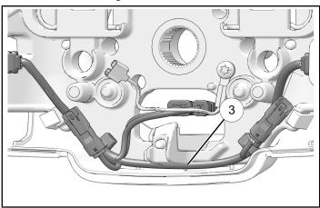
4. Insert paddle shifter wire through hole in steering wheel. Put paddle shifter ① into position.
