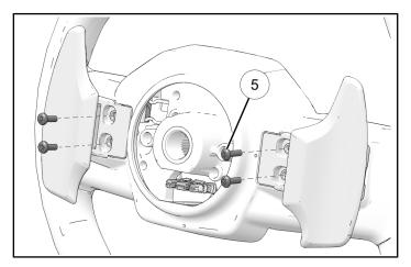
6. Connect left-hand and right-hand paddle shifter wiring harness to steering wheel harness.
