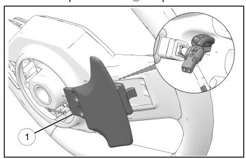
5. Install four paddle shifter screws ⑤. Torque screws to specification.
