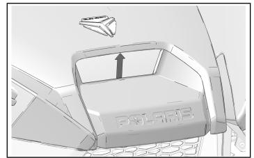
4. Pull hood upward and forward, rotating hood to a vertical position.
