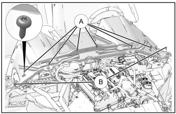
3. Torque eight screws to specification.
