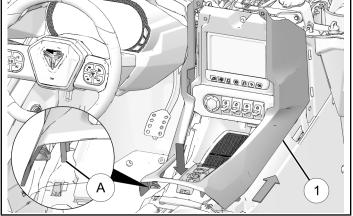
3. Attach console trim ① to upper center console using two push pin rivets ⑧.
