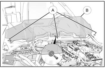
2. Torque fasteners to specification (if applicable).
