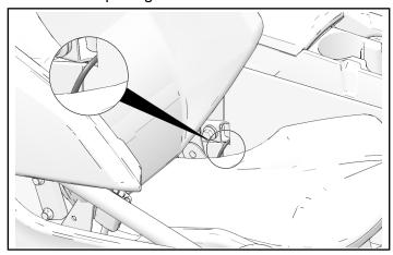
9. Connect left-hand seat harness extension 6 connector 4M to seat interior light harness 4 connector 4F.
