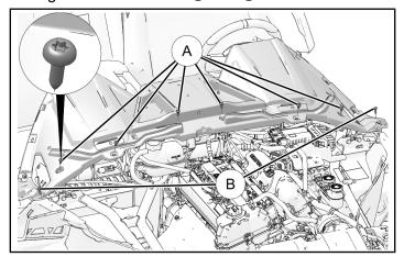
3. Torque eight screws to specification.
