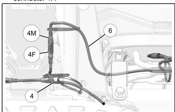
10. Connect right-hand seat harness extension ① connector 4M to seat interior light harness ④ connector 4F. Attach with cable ties ⑪.
