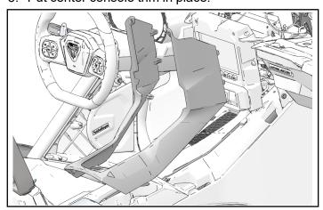
4. Install two retained push pins from center console trim.
