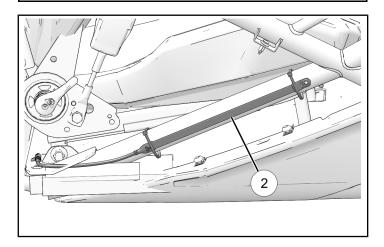
8. Remove adhesive backing paper from LED strip. Attach left-hand rocker panel LED strip ② to frame tube with cable ties.
