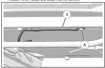
6. Remove and keep front inner left-hand seat frame screw <sup>®</sup>. Remove adhesive backing paper from LED strip. Put LED strip <sup>®</sup> on seat frame. Attach with retained seat frame screw.
