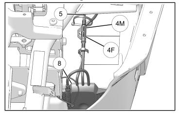
2. Put footwell interior light harness plug through firewall along existing wires. Connect harness (5) 4F to footwell LED (2) 4M. Attach with cable tie (1).
