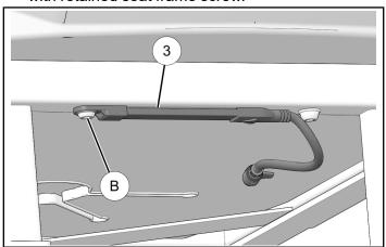
7. Remove adhesive backing paper from LED strip. Mount right-hand rocker panel LED strip ② to frame tube using cable ties.
