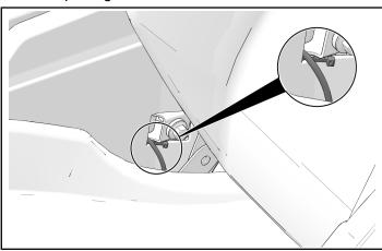
6. Connect right-hand seat harness extension ① connector 4F to right-hand seat LED ③ .
