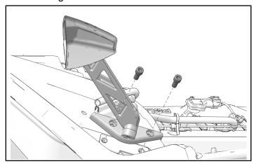
2. Torque mounting screws to specification.
