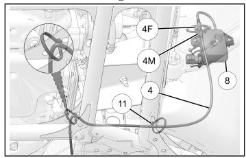
2. Put wiring harness ④ along frame rail as shown. Make sure wiring harness is routed above frame components. Attach with cable ties ⑪.
