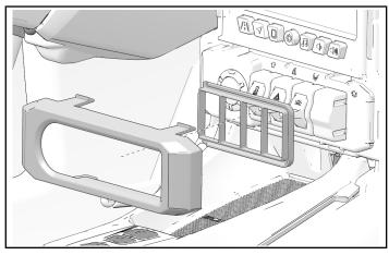
2. Put display center in place and install retained fasteners.
