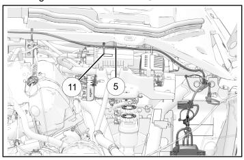
5. Put console LED wiring through firewall along existing wiring. Connect footwell interior light harness 4F to console LED ⑨ 4M.
