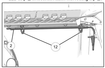
4. Put edge clips ③ in opening above steering column so LED mounts above visor closeout. Put LED strip ② with lights facing down and attach using edge clips ③.
