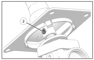
3. Attach four clips located under the shifter to install shift boot.
