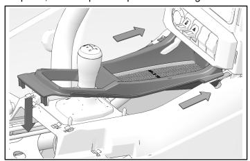
2. Tilt rear storage bin down and snap into mounts.
