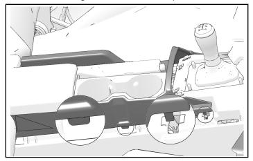
2. Attach center console trim with two retained push pin rivets (A).
