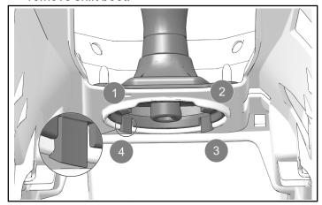
4. Lift shifter boot and remove set screw <sup>®</sup>. Remove shifter assembly from vehicle.
