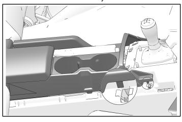
Lift end of tray assembly near shifter base to detach clips. Lift and move rearward to remove from vehicle.
