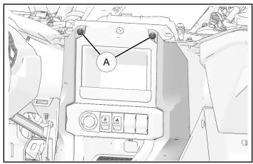
2. Lift up and pull to rear to remove center console trim. Carefully set aside.
