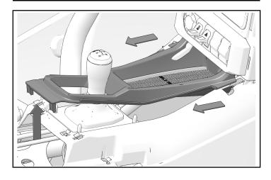
3. Detach four clips located under the shifter to remove shift boot.
