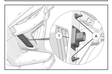
2. Locate wiring harness for lighting, clean any dirt or debris from connector and connect to LH light ① until a click is heard.
