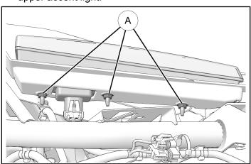
2. Remove and keep three screws ® from the back of the side marker light.
