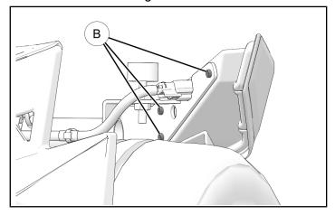
Remove and keep one screw © from the back of the side marker light. Disconnect and keep side marker light.
