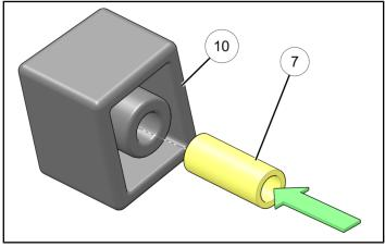
2. Rubber spacer assembly (10) into place between wind deflector (1) and top of center post (A). Install rubber O-ring (9), rubber washer (8), and screw (6) into place. Torque screw to specification.
