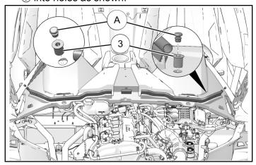
2. Install wind deflector ① by first engaging tabs and slots in front, then align mounting holes as shown with arrows.
