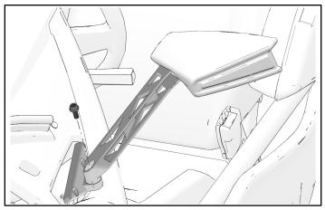
3. Remove two mounting plate fasteners and mounting plate from vehicle.
