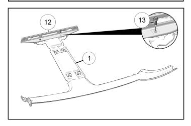
3. Set front pillars of T-top assembly ① on side mirror mount bases. Loosely install rear brace to rollover hoops with two brace fasteners ③
