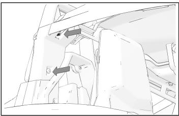
4. Close door and ensure top and bottom magnets align. Front and rear gaps may not be even when magnets are aligned.
