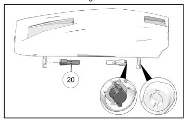
3. Hold passenger door vertical, and align hinges to T-top with smooth side facing down. Hand tighten two screws (1) per hinge. Rotate door down in a closing manner to seat hinges.
