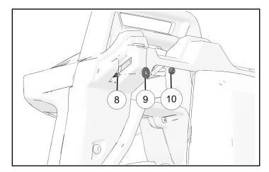
3. Secure passenger outer fin and passenger inner fin to roll hoop with two fin fasteners ①.
