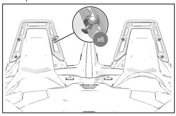
2. Attach rear brace ① to rear of T-top ① using two brace fasteners ③.
