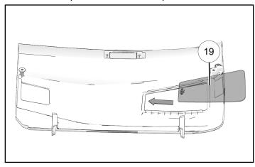
2. Align tabs of hinges ② with arms of door (shown with inset) and insert into passenger door arms with smooth side facing down.
