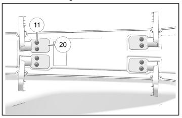
3. Close door and ensure top and bottom magnets align. Front and rear gaps may not be even when magnets are aligned.
