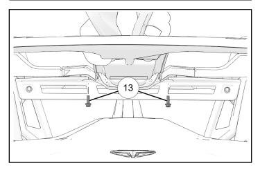
6. Tighten door hinges 20 to T-top.
