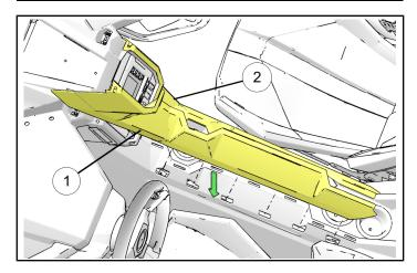
7. Install two new rivets ③ on the top center of the interior LH trim piece ① and RH trim piece ②. Firmly push rivets to ensure they seat.
