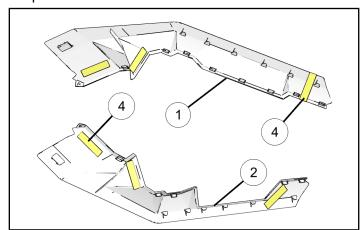
6. Starting at the back near the cup holders, install the new LH trim piece ① and RH trim piece ②. Make sure trim mounting tabs align with slots. Work all the way up to dash. Firmly push till trim pieces snaps onto center console.
