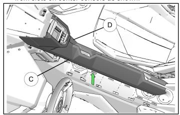
5. Clean the surface of new trim pieces ① ② and install double sided tape ④ to bottom of surface as shown. Remove the backer before installing trim pieces.
