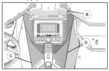
4. With both rivets out, remove LH trim piece (C) and RH trim piece (D) by starting at the top front and working back and removing trim mounting tabs from slots on center console as shown.
