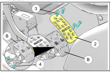
3. Tighten the screws ③ to specification using torque wrench.
