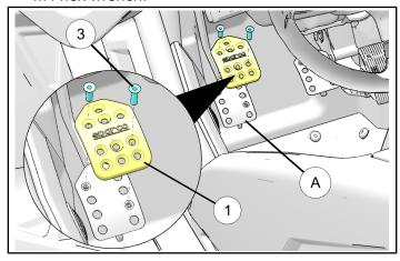
4. Tighten the screws ③ to specification using torque wrench.
