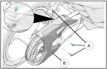
3. Install new belt guard cover ① into same mounting location using retained screws (A). Hand tighten all screws (A).
