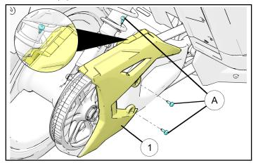
4. Using ratchet with a T40 Torx<sup>®</sup> driver tighten three screws. Torque screws to specification.
