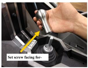
4. Using the 5mm allen wrench tighten down the set screw in the new one piece stainless steel shift knob.
