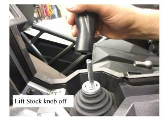
3. The next step is to slip the new one piece stainless steel shift knob into place. The set screw should be facing forward so it will make contact with the flat surface of your factory shift lever.
