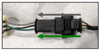
So when installing the harness, simply match the colored wires straight across from your vehicles factory wiring harness to the new conversion harness. **Grey** lines up with **Green** and **Green** lines up with **Green**.
