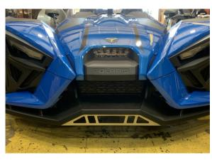
The bumper accent panel fits on the bottom of the stock bumper and adds some style and personality to your Slingshot. Installation is pretty straight forward, plan on about an hour to do the installation.
