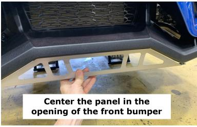
3. Line the top of the panel up with the back edge of the black plastic front bumper.
