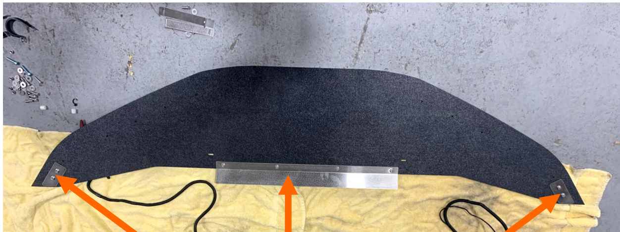
Air diverter and end clamps installed
