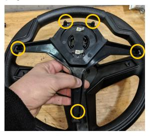
2. 2. With the horn button assembly out of the way you will see the nut holding the steering wheel onto the steering shaft. Use a 24mm socket to remove the nut.
