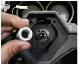
In some cases the steering wheel will pull off just using your hands. Most of the time though, a steering wheel puller is necessary. Steering wheel pullers are available online through several sources, including Slingmods.com.
